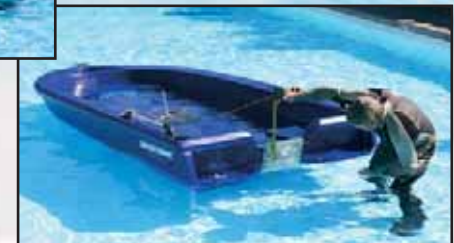
Testing procedure with boat fully swamped.
