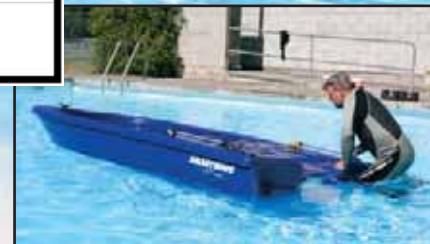
Testing procedure with boat fully swamped.
